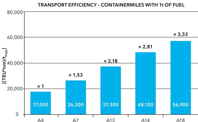
While the previous vessels were all standard shipyard designs that only underwent limited optimisation and were trimmed for the common high operational speeds at that time, the new vessels of 14,500 TEU (A14 class) and 18,800 TEU (A18 class) were developed for economy and best fuel consumption by UASC with their consultant TECHNOLOG and the tendering shipyards, later the selected builders HHI, in successful partnership. These newbuilds have the following particulars:
